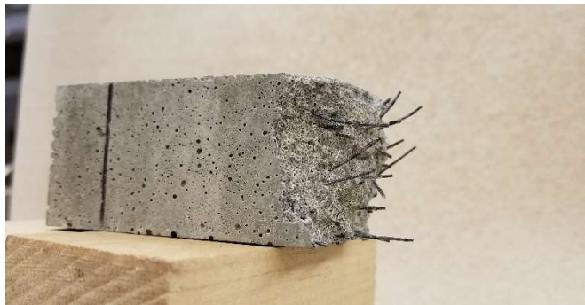
Figure 6-5 Fiber Orientation Distribution: Horizontal Biased
