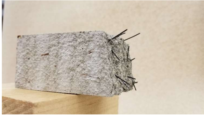
Figure 6-3 Fiber Orientation Distribution: Vertical Biased
