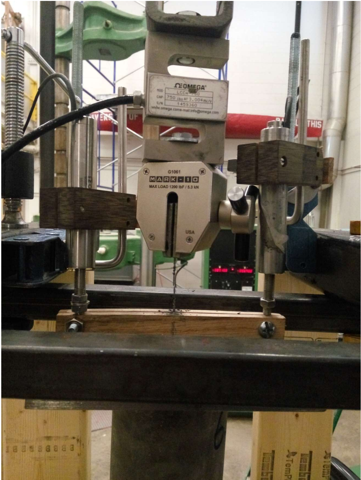
Figure 4-4 Typical Fiber Pull-Out Specimen Just Prior to Test
