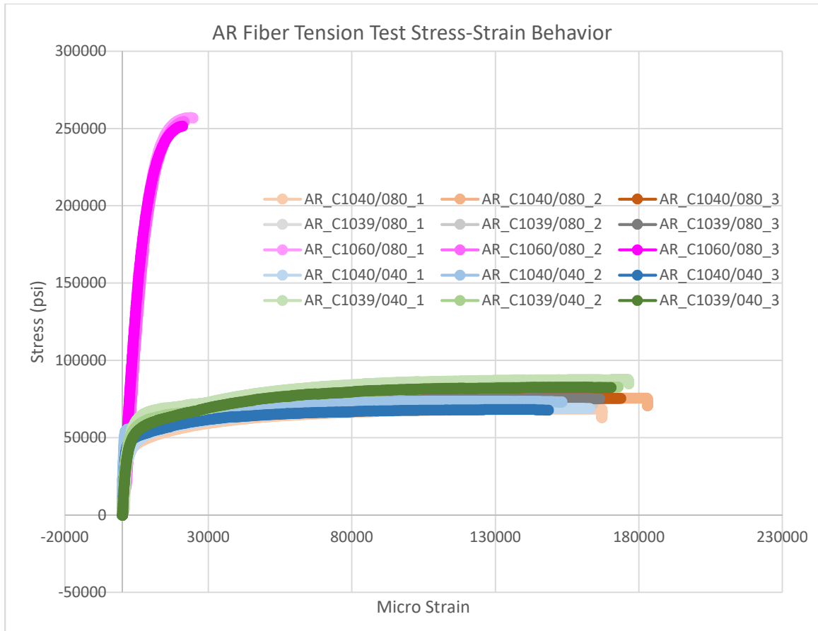
Figure 5-1 Tension Test Results of As Received Fibers (Stress in psi, Strain in microstrain)
